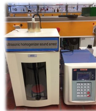
Ultrasonic probe 200 W Exfoliation of layered materials
