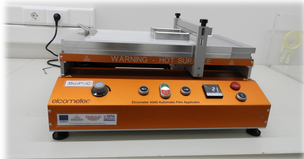
Automatic wet-film applicator (1-50 mil), Temp. 180 °C
