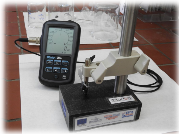
Thickness meter (0.1 \mu\text{m} )
