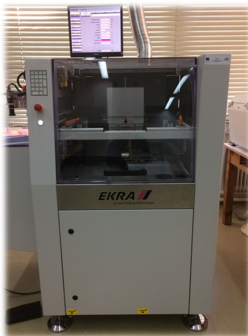
Screen-printer with laser automatic alignment
