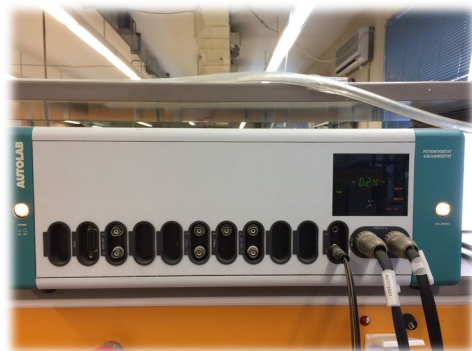
Frequency Response analyzer Impedance Spectroscopy
